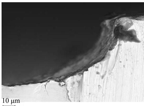
Fig. 10. SEM images of (top) an uncoated channel (200×) and (bottom) an Ag/alumina coated channel (1000×).
