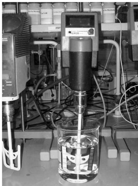
Fig. 6. Impregnation of the microplates using a conventional stirrer.
